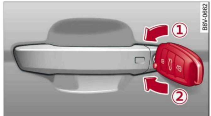
Fig. 26 Driver's door lock
