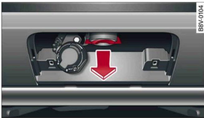
Fig. 85 Area below rear bumper: Pulling out plug
