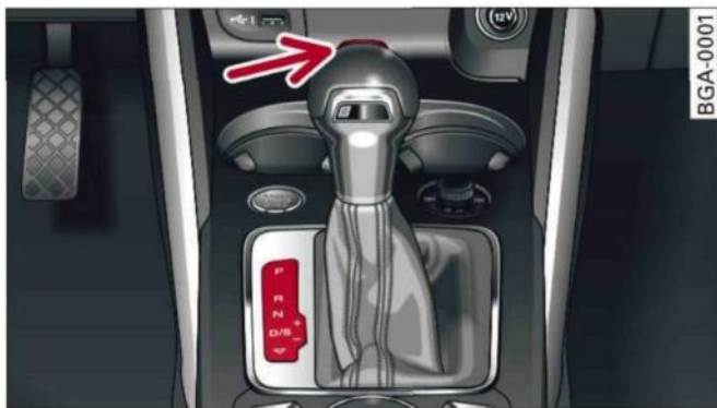
Fig. 77 Detail of the centre console: Selector lever with interlock button
