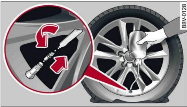
Fig. 258 Tyres: Filling the tyre
