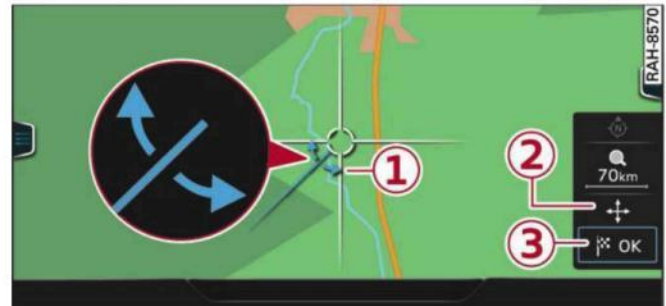
Fig. 173 Moving the crosshairs (MMI control console with rotary pushbutton with joystick function)
