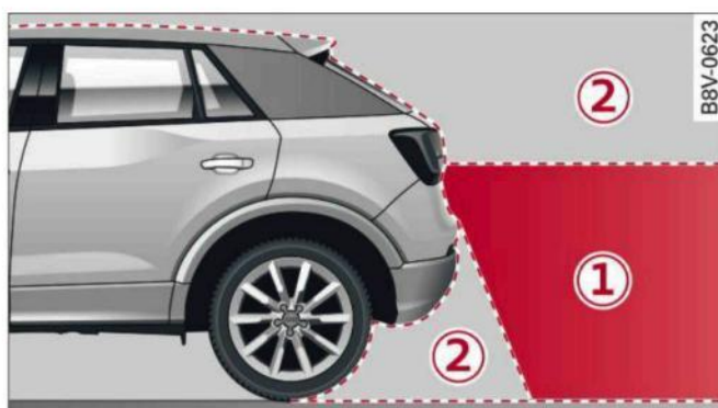
Fig. 128 ①: Area covered by the reversing camera; ②: area NOT covered by the reversing camera (example)
