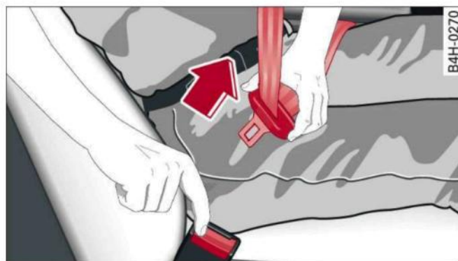
Fig. 225 The latch plate of the belt springs out of the buckle
