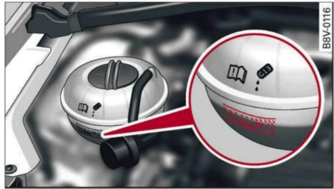
Fig. 248 Engine compartment: Markings on coolant expansion tank
