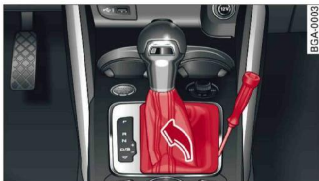
Fig. 80 Selector lever: Removing the boot
