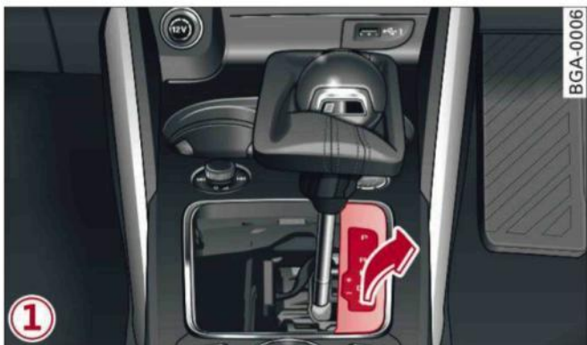
Fig. 82 Selector lever: Removing the boot
