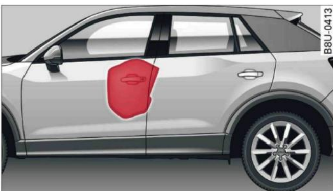
Fig. 233 Side airbags in inflated condition
