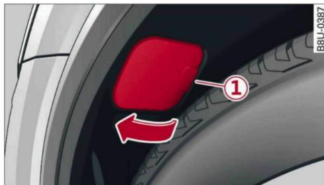
Fig. 286 Wheel housing liner: Access to daytime running light and dipped headlight bulbs
