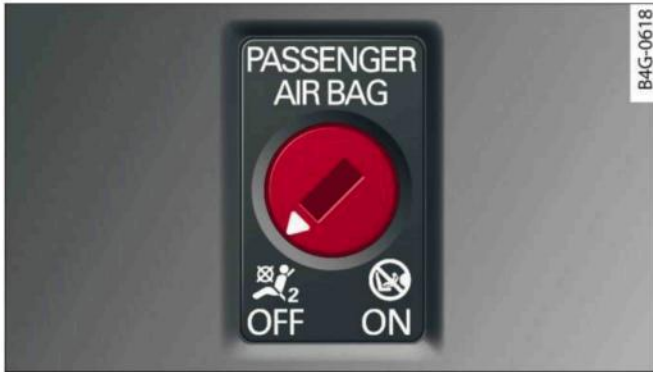
Fig. 236 Glove box: Key-operated switch for deactivating front passenger's airbag
