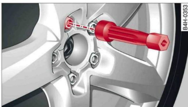
Fig. 264 Wheel: Hexagonal socket for turning wheel bolts
