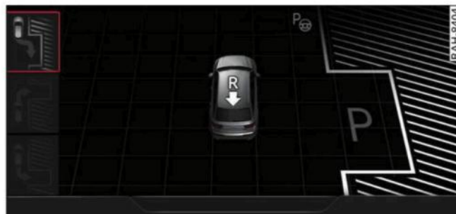
Fig. 138 Infotainment system: Prompt to continue reversing (example: parking parallel to the roadside)
