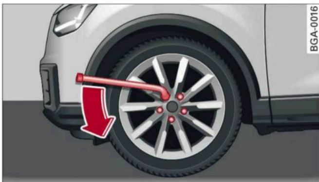
Fig. 261 Wheel: Loosening the wheel bolts
