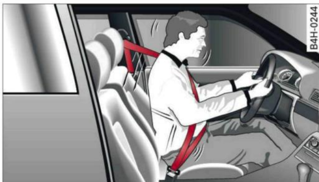
Fig. 215 Driver with correctly positioned seat belt – good protection if the brakes are applied suddenly
