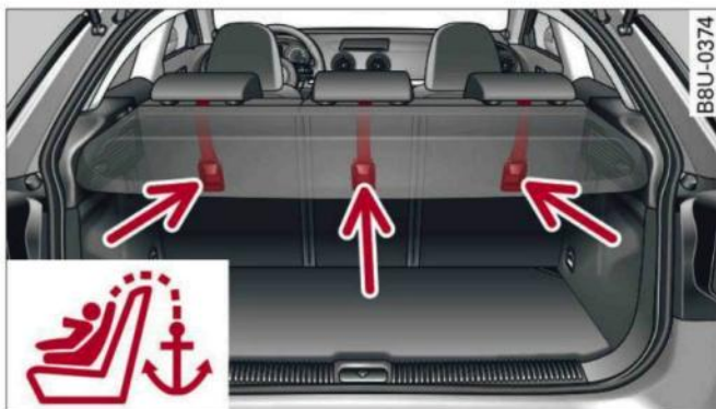
Fig. 212 Rear backrest: Top tether anchorages (version 1)
