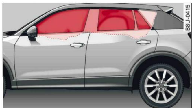
Fig. 235 Head-protection airbags in inflated condition (example)
