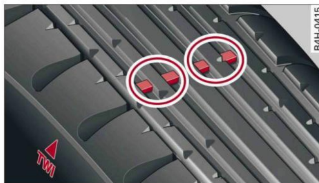
Fig. 252 Tyre tread: Tread wear indicators
