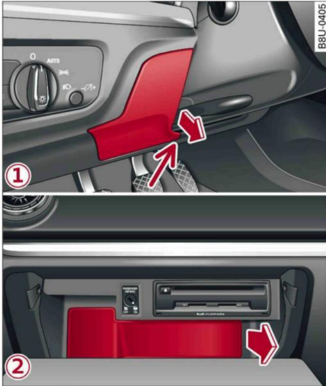
Fig. 275 ① Steering column area (LHD vehicles): cover, ② Glove box (RHD vehicles): cover
