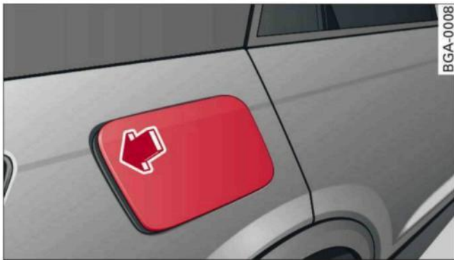
Fig. 238 Vehicle as seen from the rear right: Opening the fuel tank flap
